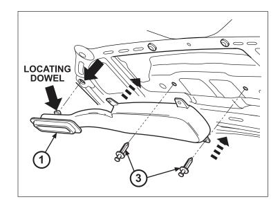
11. Use Ram Air Scoop (1) to locate mounting holes. Using a hammer and hole punch, punch a starter hole in the frame rail in each Ram Air Scoop mounting hole for drilling final mounting holes.
