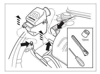
3. Loosen four M6 bolts and remove airbox cover using a 10mm socket, save for reinstallation.
