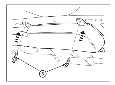
14. Install new Ram Air grill (2) into hood, back side in first rocking back and forth until a click is heard on each side. This will ensure a secure fit for the Ram Air grill.
