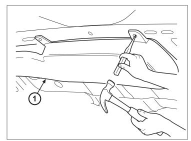
CAUTION: When drilling mounting holes into the aluminum hood, ensure that you mark the drill bit first with black tape exactly 1/2" down from the tip to ensure that drill bit does not penetrate hood surface.
