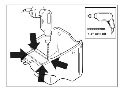
NOTE: When cutting out airbox access cover, ensure you cut on the outer edge of scribe marks.
