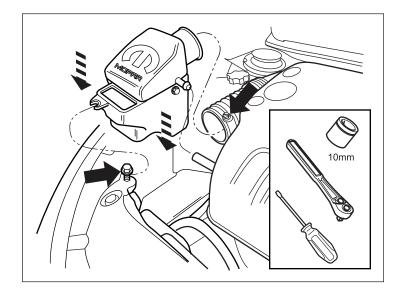
8. Using a phillips screwdriver disengage two tabs through access holes and, pry original hood vent. Discard hood vent.
