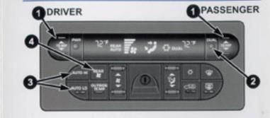
Adjust driver "TEMP" 1 to the desired temperature. (Try 72° to start).
